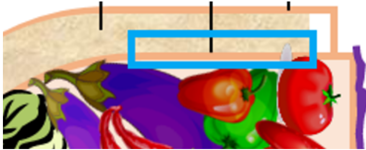
Fig. 5: Experiment models the area in the blue box, a section of the pot-in-pot refrigerator from Fig. 3 turned 90° clockwise.
