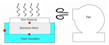
**Figure 6:** Schematic of experimental setup with a fan blowing over the water-soaked material. Temperature sensors (red dots) are placed to record the temperature at the top and bottom of the block and the ambient air. These are connected to Logger Pro data collection units (not pictured).
