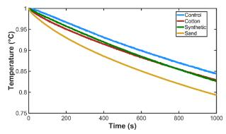
**Figure 8:** Ratio of temperature at time *t* to initial temperature over the data collection period. Note the improved cooling by placing a wet material on the block.
