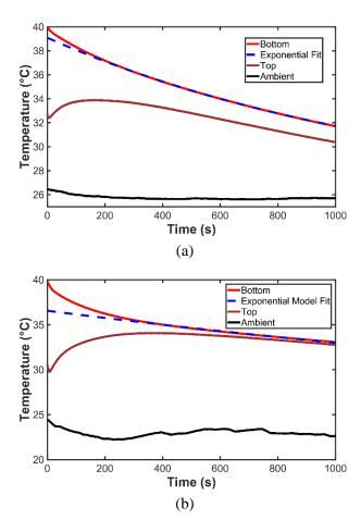
**Figure 9:** (a) Sand with wind speed of 3.2 m/s. (b) Sand with wind speed of 0 m/s. Notice the difference in the fit curve towards the beginning of the data collection period.
